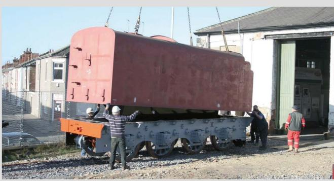
Fifteen years ago we were also moving tender tanks around the yard at DLW I. This is *Tornado's* being fitted to its frames.
