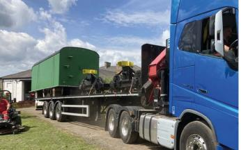
The tender tank sees the light of day for the first time in a while, and together with its accommodation bogies, is loaded at DLW1.
