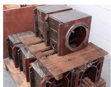
Terry Graham and I ventured to Howco in Irvine to see progress on the cylinder block and to deliver some more items required to blank off all the holes to enable the hydraulic test to be carried out. By and large the results are satisfactory - almost everything we tried on the cylinder block fitted - we had to bring the release valve adapters for the cylinder covers back for a bit of thread easing. TCC
