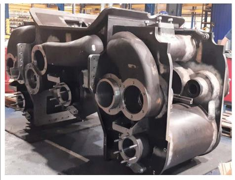
Trial fitting covers and blanks to rear of cylinder block.
