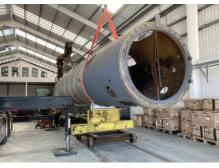
Above and right: With the tender tank moved, *Tornado's* boiler was extracted from the old works, trundled through Darlington and off-loaded at DLW2.
