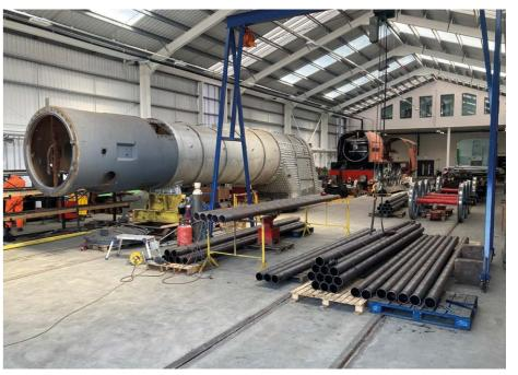
Flue tubes and boiler in the new works.
